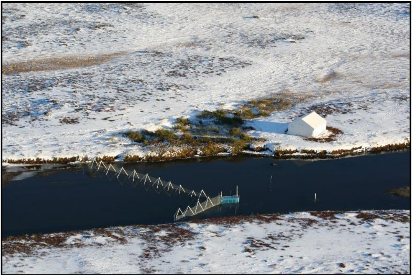
Figure 1. Counting fence used to monitor Arctic charr during upstream migration in August and September 2016, on Voltz River, Aupaluk, Nunavik.
