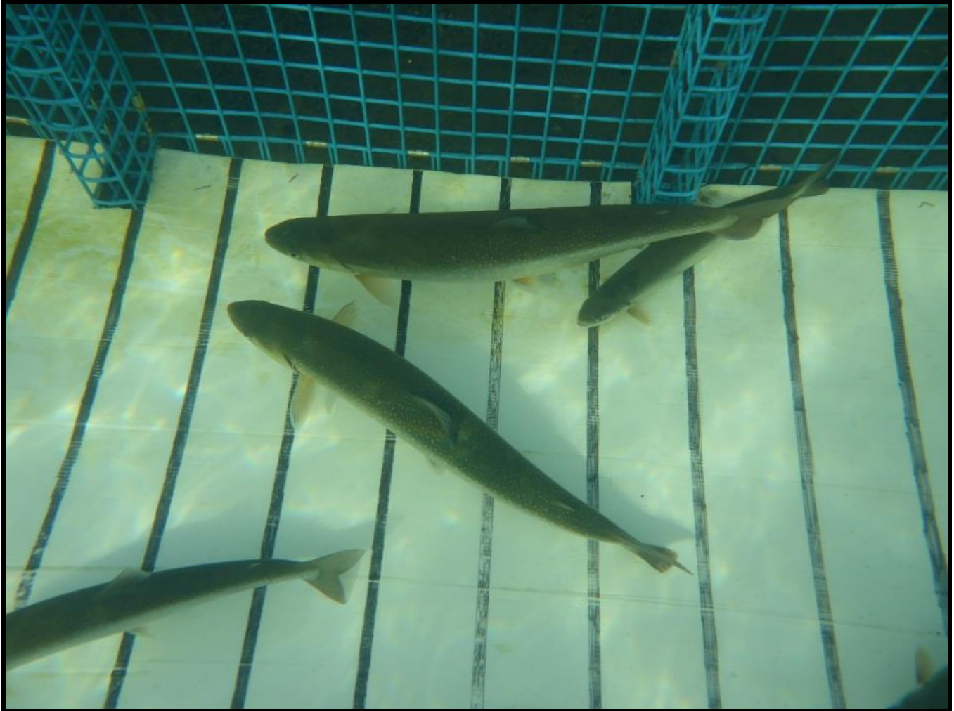
Figure 2. Measuring lines 10 cm apart on the floor of the holding cage, used to estimate the size of the Arctic charr before they were released upstream.
