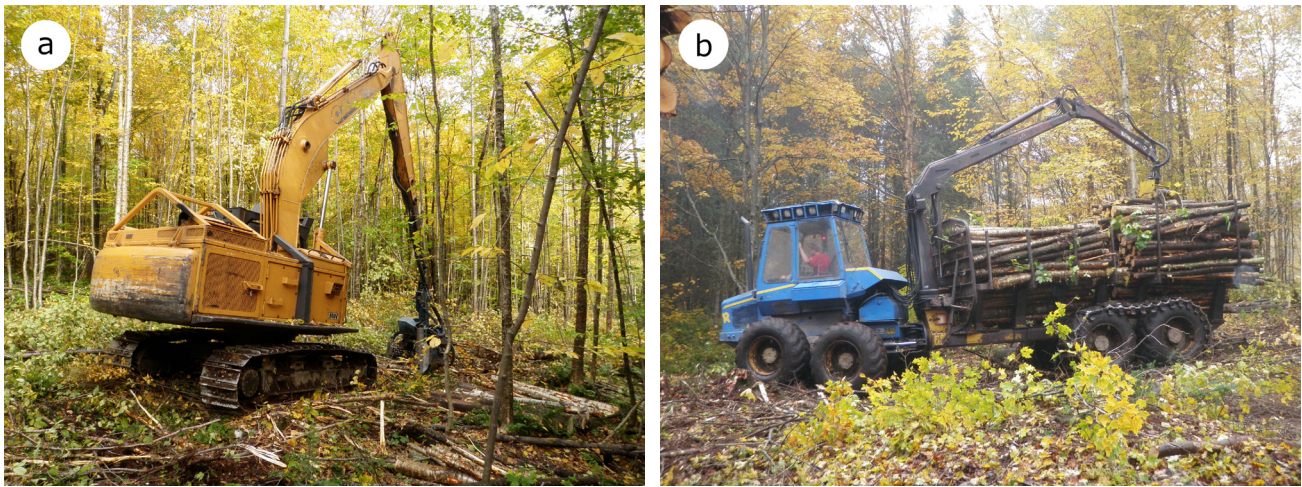
Figure 2.—Machinery used for harvesting: (a) harvester with a processing head; (b) forwarder. Courtesy photo by François Guillemette/MFFP, used with permission.
