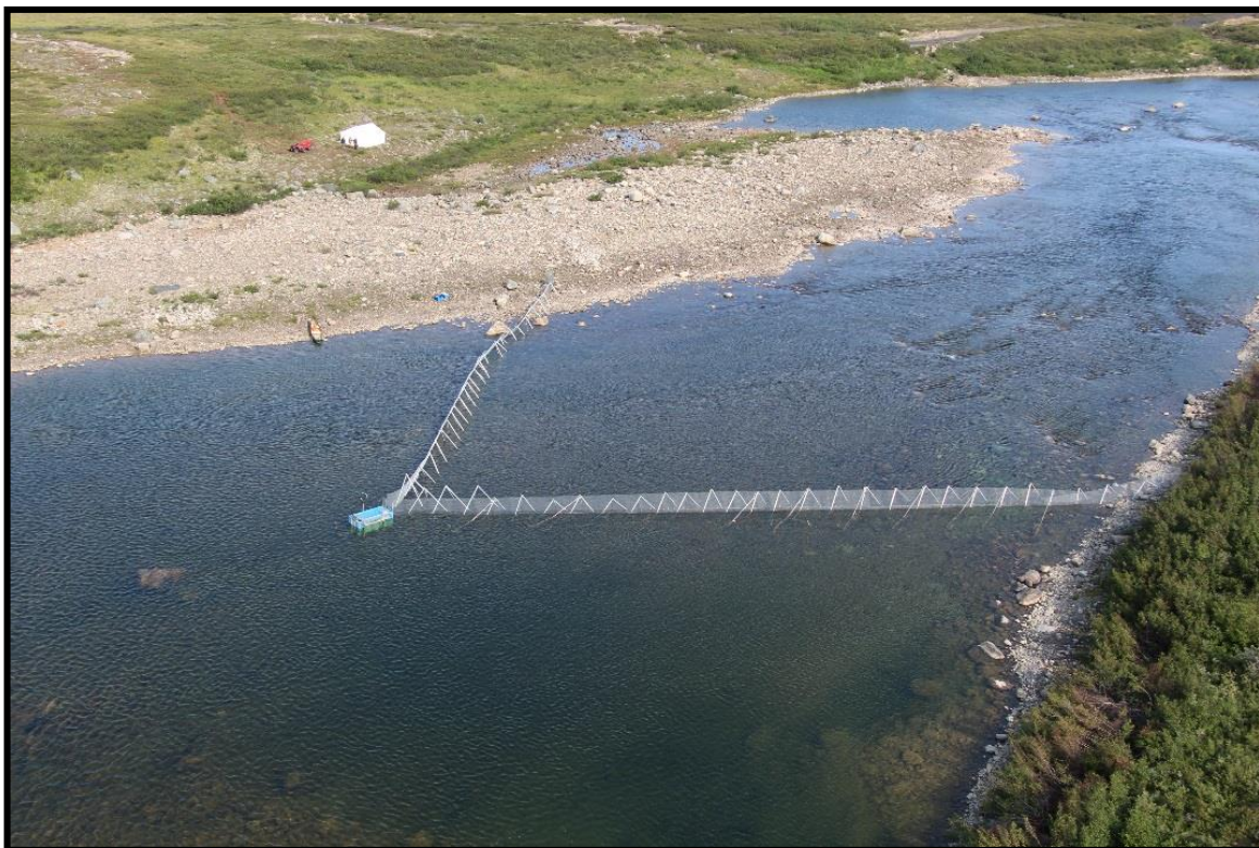
Figure 1. Counting fence used to monitor Arctic charr during upstream migration in August and September 2017 on the Bérard River, in Tasiujaq, Nunavik. A canoe (visible in the photo) provided access to the retention cage from the riverbank. A tent, also visible in the photo, was used to protect the temporary laboratory.
