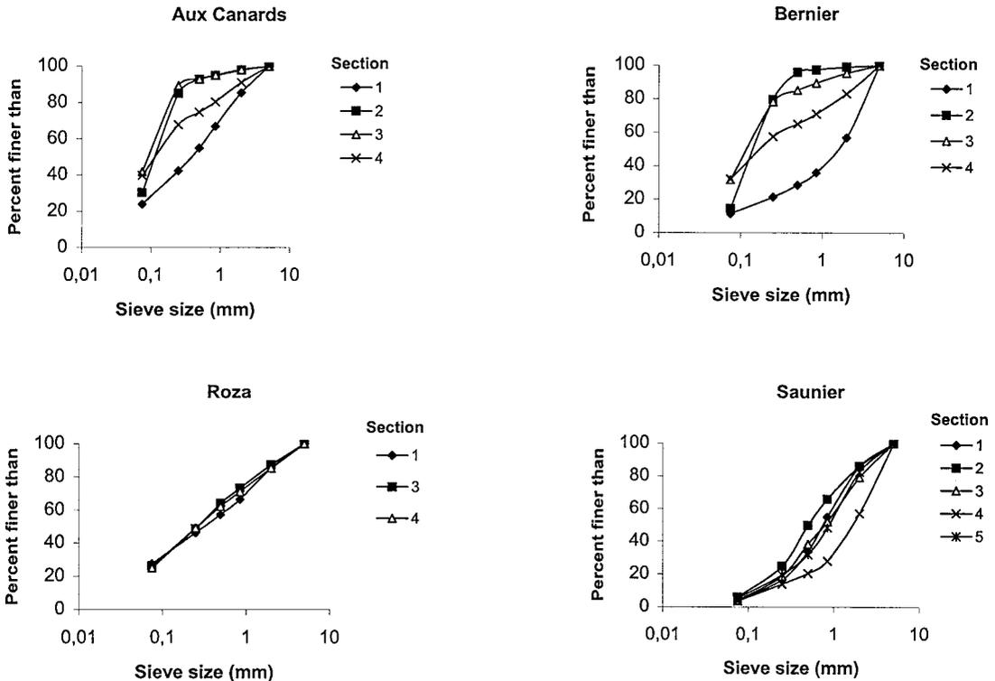
FIGURE 3.—Grading curves of fine sediment (diameter  $< 5$  mm) accumulated in the SÉDIBAC 45 in the first autumn (2000) following culvert construction, for each study section of the Aux Canards, Bernier, Roza, and Saunier streams on the Laurentian Shield, Québec.
