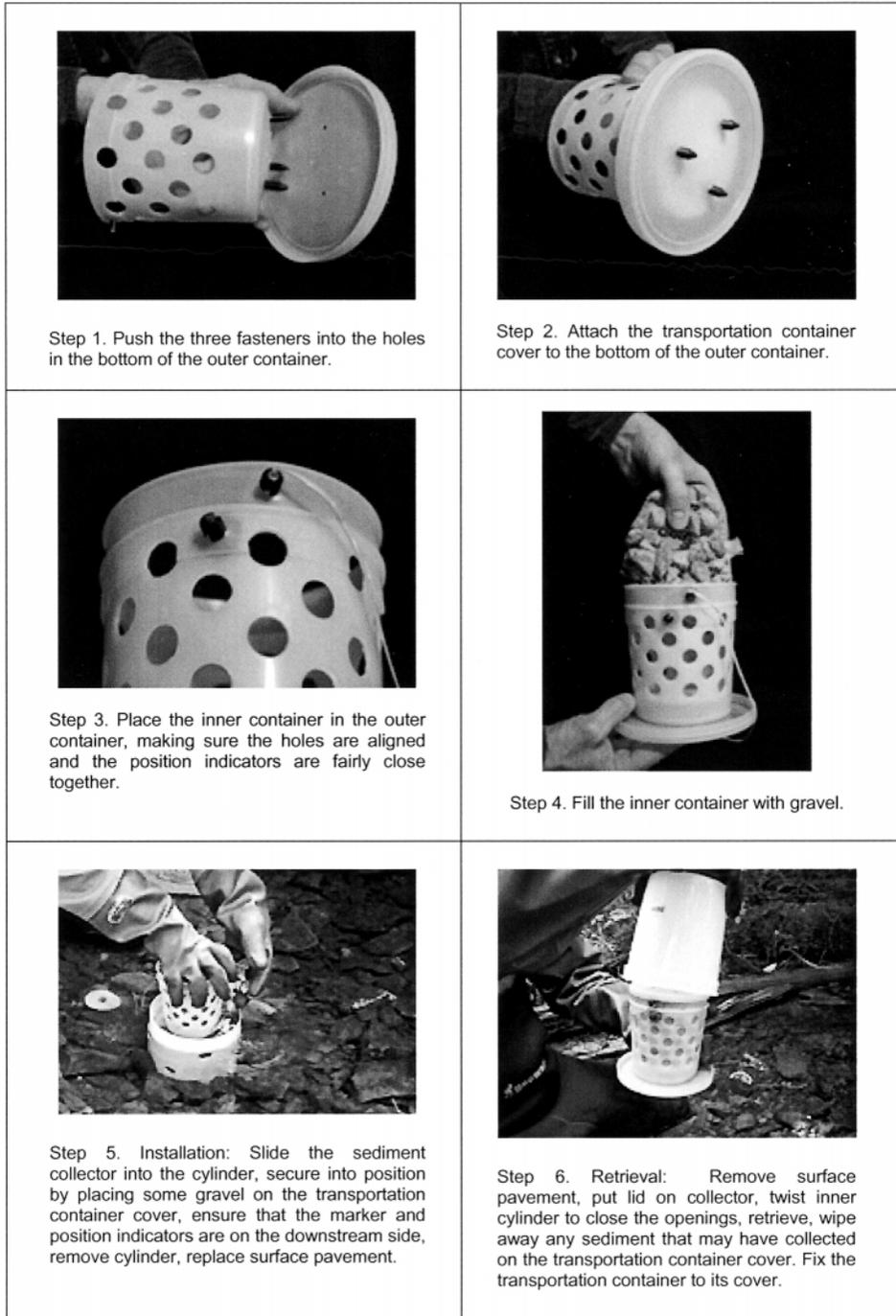
FIGURE 2.—Six steps for the use of the SÉDIBAC 45 sediment collector, from mounting to retrieval.
