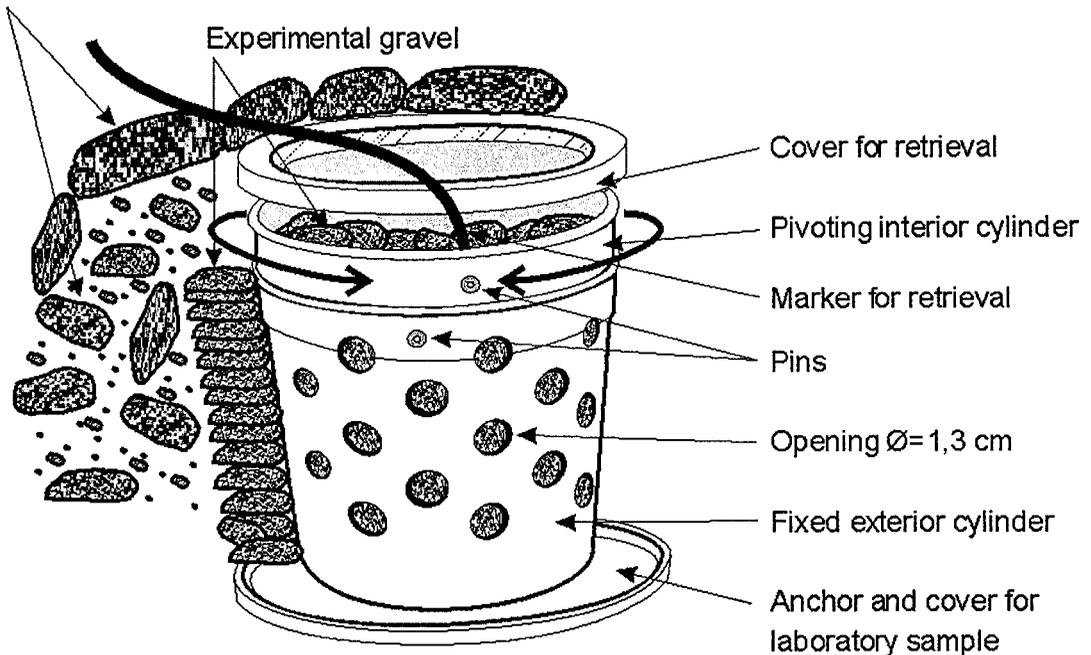
FIGURE 1.—The SÉDIBAC 45 sediment collector and its components (patent pending, Bio-Innove, Inc. 2002). The collector was used to sample sediment accumulation following culvert construction in four Laurentian Shield streams, Québec.
