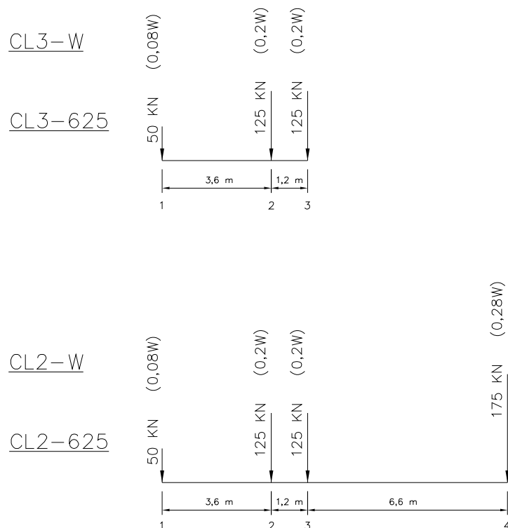
Figure 2 - Configurations CL-W et CL-625
