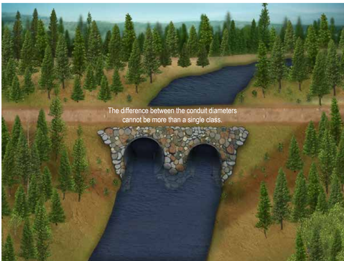
Figure 102A Culvert with parallel conduits of different diameters
