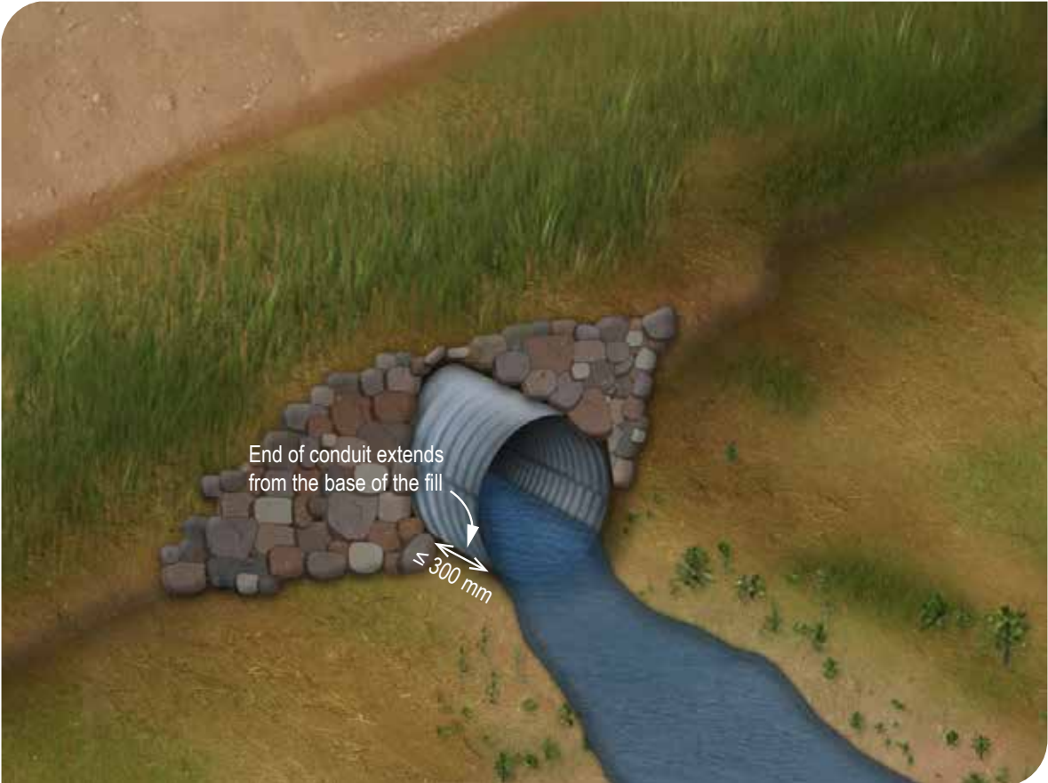
Figure 100A End of a conduit or arch extending from the base of the embankment
