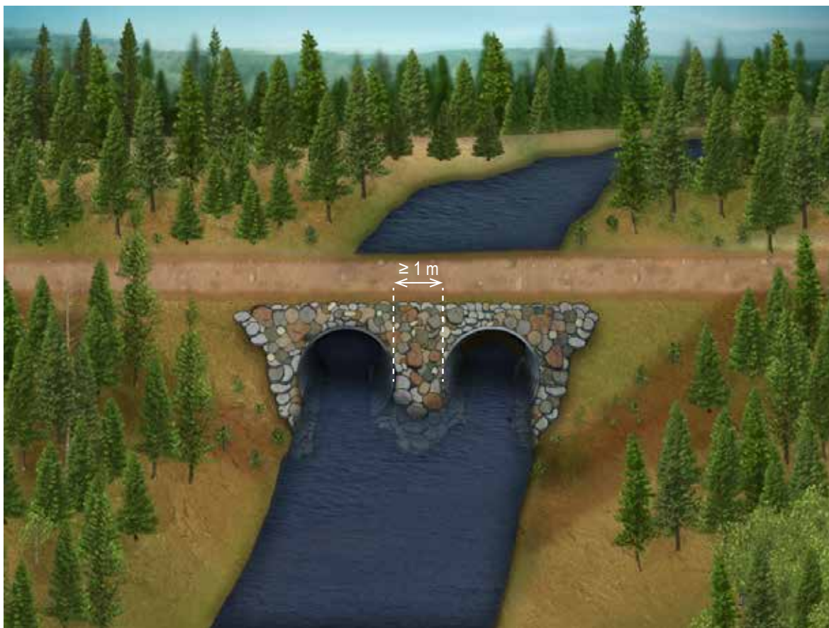
Figure 102B Distance between the conduits of a culvert with parallel conduits
