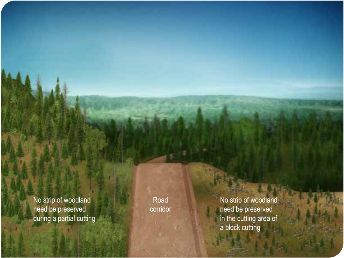
Figure 8E Block cutting and partial cutting along a road corridor
