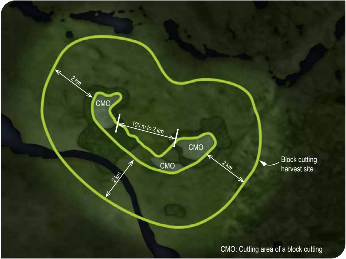
Figure 2B Diagram showing a block cutting harvest site
